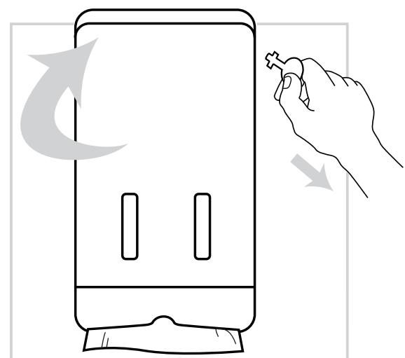
6. Remove key from lock and firmly close front lid.
