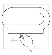
When left roll is empty, slide lever at base of dispenser left until it locks in place.
