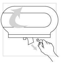
5. Remove key from lock and firmly close front lid.
